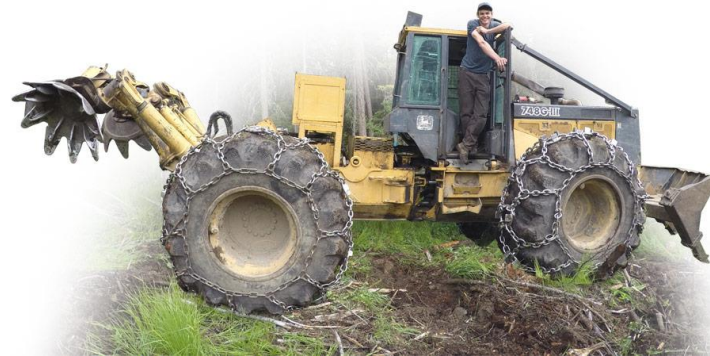
FORWARDER WITH TRENCHER
